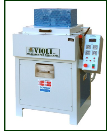
Low-melting alloy emptying machine VM/SCG
