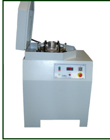
Low-melting alloy centrifugal injector VM/MIV
