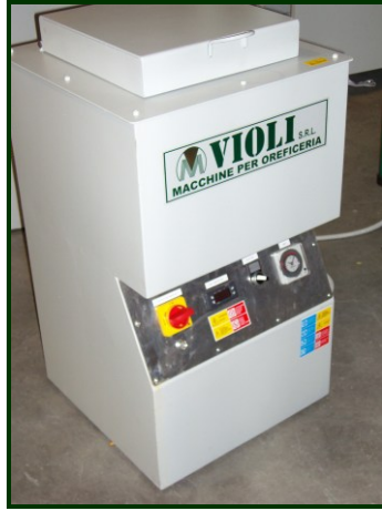
Eutectic low-temperature melting furnace VM/VS
